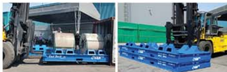
● ISO Fork Lift Pocket (@ Rear & Sides)
