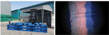
● Paint 3 Layers (30/40/30 D.F.T 110 μm)
